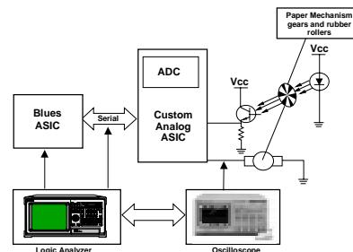
The system was partially verified as analog with the oscilloscope. The logic analyzer de-serialized the data stream and on the ASIC emulator we were able, with the logic analyzer, to verify the completed feedback path.
