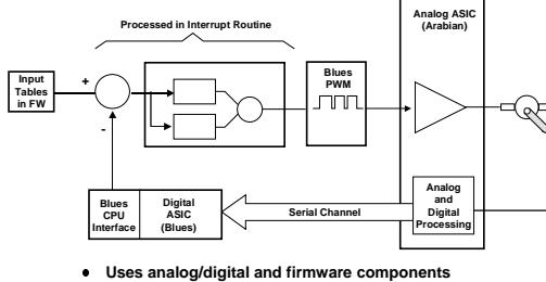
Verifying that the components are being re-combined correctly is a complex task. It is necessary to time correlate analog, serial digital and firmware tasks.
